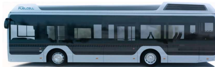
Caetano: Hydrogen bus with Toyota fuel cell
