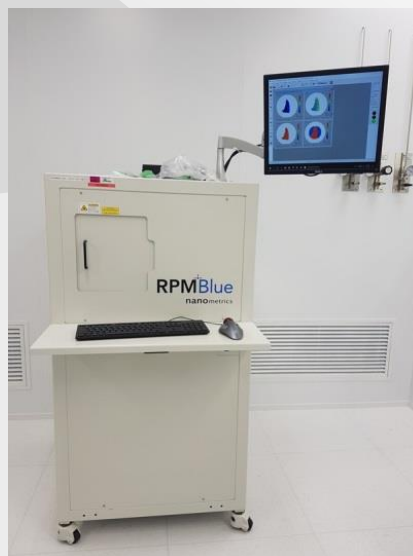
Photoluminescence (PL) mapping (0.3-2.6 \mu\text{m} )
