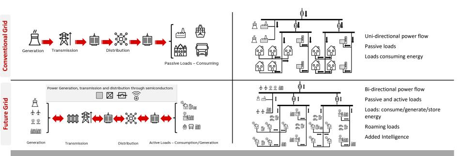
Evolving into electronically controlled and protected power grid - here comes Digital & Power Electronics
